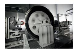
In order to continuously optimise our inspection and test capacities, we use a drum test rig for wheels and castors.
